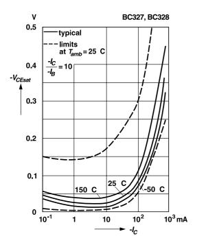
Collector saturation voltage versus collector current
