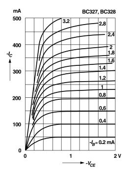
Common emitter collector characteristics
