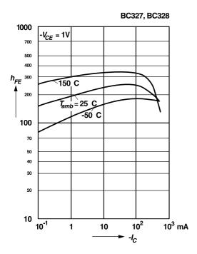
Common emitter collector characteristics
