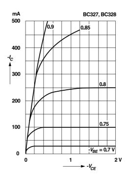
Common emitter collector characteristics
