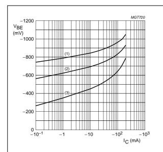
**BC857CW**;  $V_{CE} = -5 \text{ V}.$
