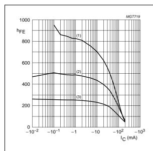
**BC857CW**;  $V_{CE} = -5 \text{ V}.$
