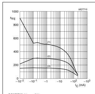
**BC857BW**;  $V_{CE} = -5 \text{ V}.$
