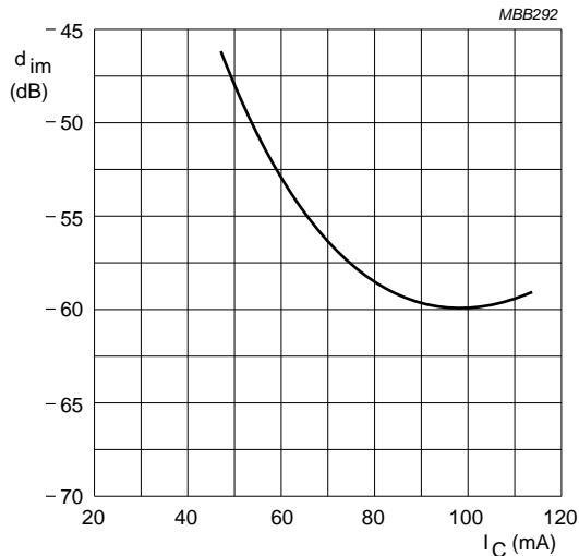
$V_{CE} = 10$  V;  $V_o = 900$  mV;  $T_{amb} = 25$  °C;
