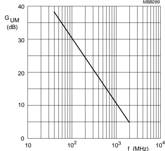
$I_C = 100\text{ mA}; V_{CE} = 10\text{ V}; T_{amb} = 25^\circ\text{C}.$
