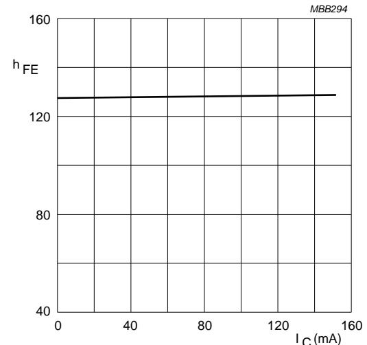
$V_{CE} = 10$  V;  $T_j = 25$   $^\circ\text{C}$ .
