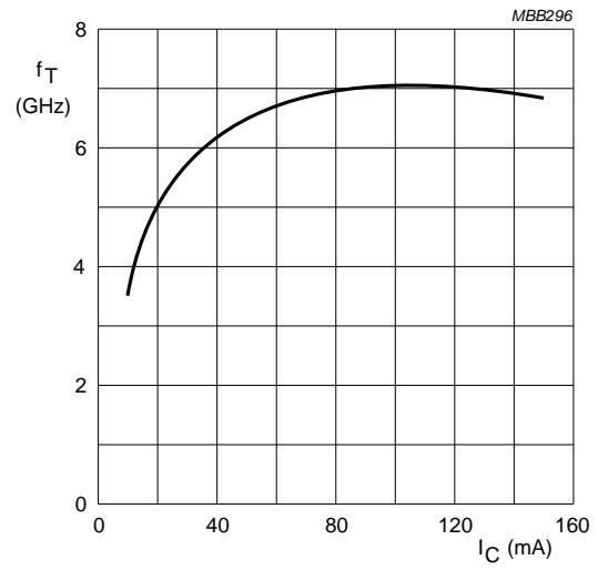
$V_{CE} = 10$  V;  $f = 1$  GHz;  $T_{amb} = 25$   $^\circ\text{C}$ .
