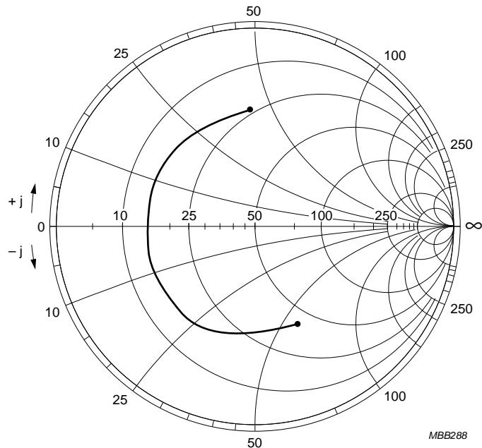
$I_C = 100 \text{ mA}; V_{CE} = 10 \text{ V}; T_{amb} = 25^\circ \text{C}; Z_o = 50 \Omega..$
