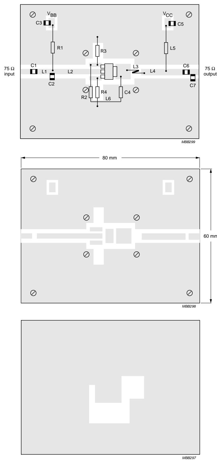
Fig.3 Intermodulation distortion test printed-circuit board.
