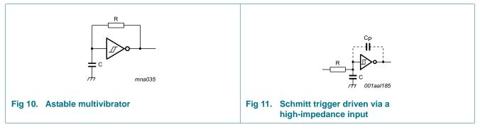
If a Schmitt trigger is driven via a high-impedance (R > 1 k $\Omega$ ), then it is necessary to
