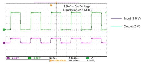
Figure 12. Translation Up (1.8 V to 5 V) at 2.5 MHz
