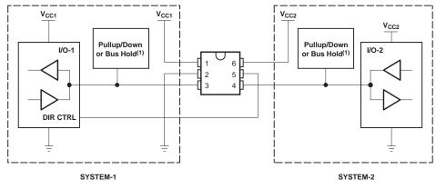
Figure 13. Bidirectional Logic Level-Shifting Application
