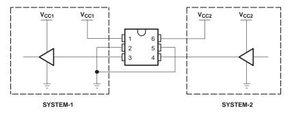
Figure 11. Unidirectional Logic Level-Shifting Application
