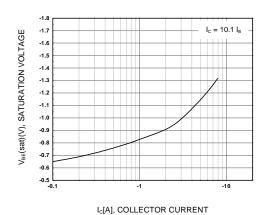
Figure 2. Base-Emitter Saturation Voltage
