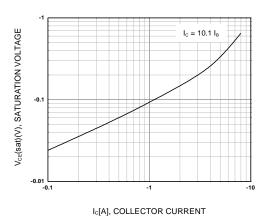
Figure 3. Collector-Emitter Saturation Voltage
