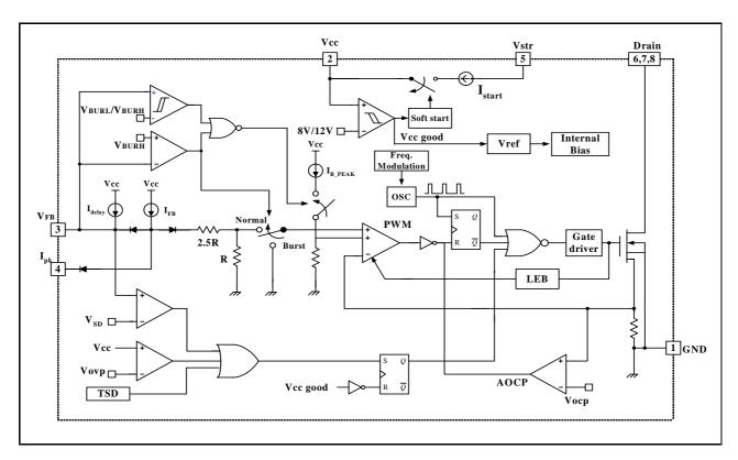
Figure 2. Functional Block Diagram of FSDx321
