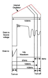
Figure 11. Frequency Modulation Waveform for FSDH321
