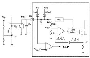
Figure 5. Pulse width modulation (PWM) circuit
