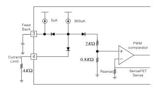
Figure 12. Peak current adjustment
