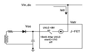
Figure 4. High voltage current source
