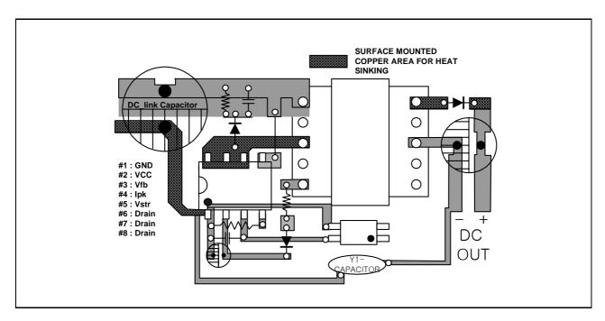
Figure 13. Layout Considerations for FSDx321 using 8DIP
