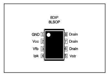
Figure 3. Pin Configuration (Top View)
