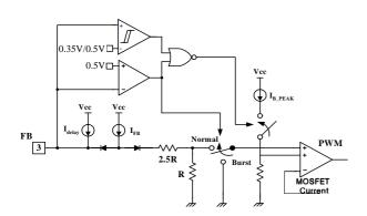
Figure 9. Circuit for Burst operation
