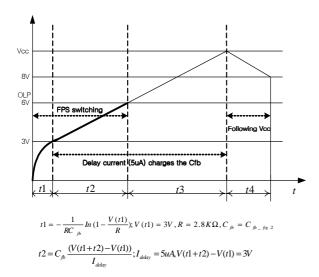
Figure 6. Over load protection
