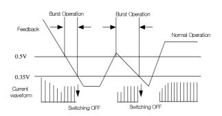
Figure 10. Circuit for Burst Operation
