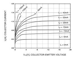
Figure 1. Static Characteristic
