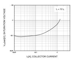
Figure 3. Collector-Emitter Saturation Voltage
