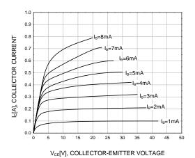
Figure 1. Static Characteristic
