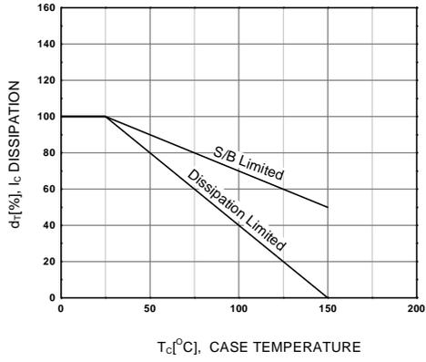
Figure 7. Derating Curve of Safe Operating Area
