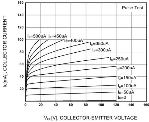
Figure 1. Static Characteristic
