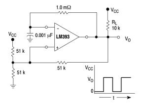
Figure 10. Free-Running Square-Wave Oscillator
