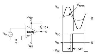
$V_{in(min)} \approx 0.4$  V peak for 1% phase distortion ( $\Delta \Theta$ ).
