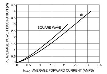
Figure 9. Power Dissipation
