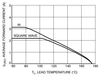
Figure 7. Current Derating, Lead
