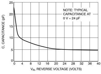
Figure 5. Typical Capacitance
