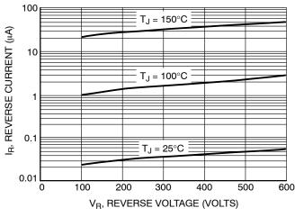
Figure 1. Typical Reverse Current
