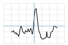
Oscilloscope setting: Vertical 50mV/div Horizontal 50µs/div
