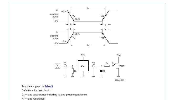
Fig 13. Test circuit for measuring switching times
