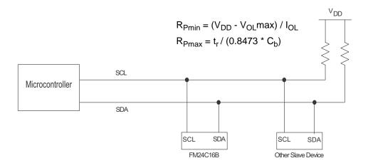
Figure 2. System Configuration using Serial (I<sup>2</sup>C) nvSRAM
