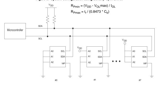
Figure 3. System Configuration using Serial (I<sup>2</sup>C) nvSRAM
