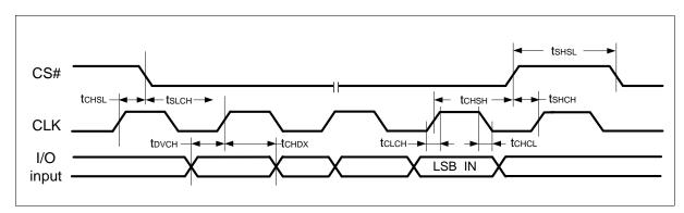
Figure 18 Serial Input Timing
