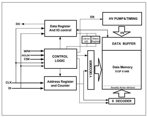
Figure 1 Block Diagram
