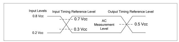
Figure 16 AC Measurement I/O Waveform
