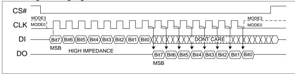
Figure 2 The difference between Mode 0 and Mode 3
