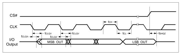
**Figure 17 Serial Output Timing**
