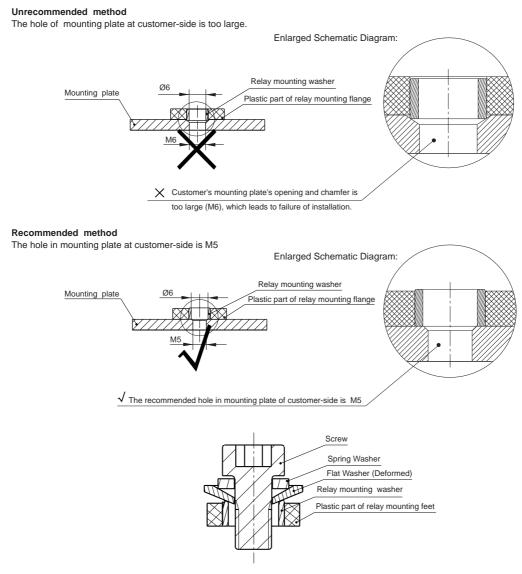
When use M5 screw, the thickness and strength of the washer needs to be guaranteed or it may deform and burst the cover.
