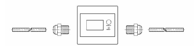
Materials : Sensor Body : Acetal Copolymer, TICONA M90 Turbine : Acetal Copolymer, TICONA M90 Stick of Turbine : #304 Stainless Steel O-Ring : EPDM Rubber Housing : ABS resin
