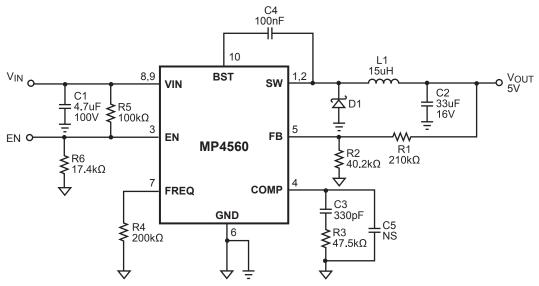
Figure 4—5V Output Typical Application Schematic
