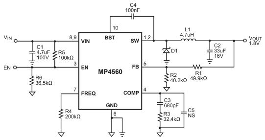
Figure 3—1.8V Output Typical Application Schematic
