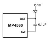
Figure 2—External Bootstrap Diode
