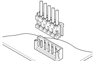
This, the thinnest, 2.5mm pitch connector, is 8.1mm in height after mounting and 3.8mm in width. It is designed to meet the demand for the high-density connection of internal wires to printed circuit boards. It is compact, highly reliable and low in cost.
