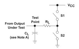
Figure 2. Load Circuit
