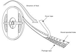
Fig. 16 - TGS8100 packaging structure
