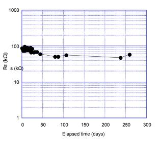
Fig. 11 - Long-term stability (continuous energizing) in clean air
