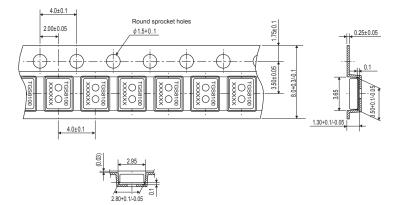
Fig. 17 - Dimensions of packaging tape
