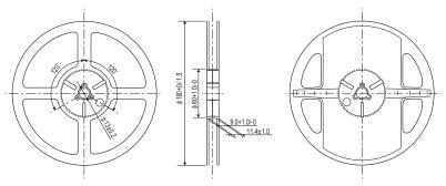
Fig. 18 - Dimensions of tape reel
