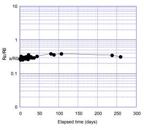
Fig. 12 - Long term stability (continuous energizing) in 10ppm H2
