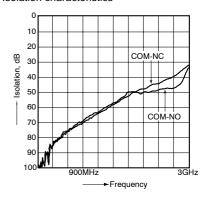
1-(2). High frequency characteristics (Impedance  $50\Omega$ ) (Standard PC board terminal)
