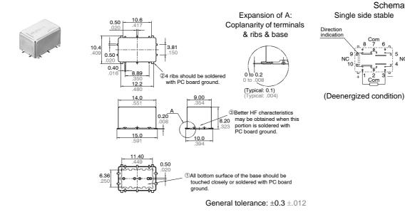
Schematic (Top view) Single side stable 2 coil latching
