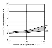
7-(2). Electrical life test (Lamp load)
