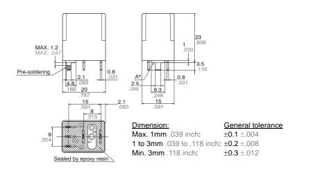
\* Dimensions (thickness and width) of terminal specified in this catalog is measured before pre-soldering.
