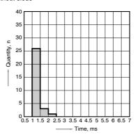
8-(1). Electrical life test (Motor free) Sample: CM1aF-R-12V, 6pcs. Load: Cooling fan motor actual load (free condition) Switching frequency: (ON:OFF = 2s:6s) Ambient temperature: Room temperature
