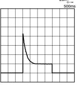
8-(2). Electrical life test (Halogen lamp load)
