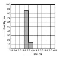
6. Distribution of release time Sample: CP1-12V, 100pcs Ambient temperature : 20°C 68°F \* With diode
