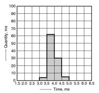
7-(1). Electrical life test (at rated load)
