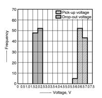
7-(1). Electrical life test (at rated load) Sample: JJM1-12V
