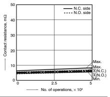
7-(4). Electrical life test (Lamp load) Sample: JJM1-12V, 6pcs. Load: 27W+21W, min. 4A (steady), Lamp actual load Operating frequency: ON 2s, OFF 13s Ambient temperature: Room temperature
