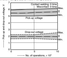
7-(2). Electrical life test (Motor free) Sample: JJM1-12V, 6pcs. Load: 5A, Inrush 25A, Brake current 18A 14V DC, Power window motor load (Free condition). Operating frequency: (ON : OFF = 0.5s : 9.5s) Ambient temperature: Room temperature
