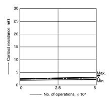
4-(3). Electrical life test (Motor load)
