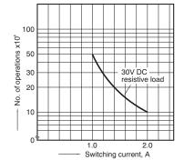
3. Mechanical life Tested sample: TX2-5V, 10 pcs. Operating speed: 180 cpm
