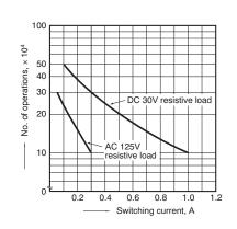
3. Mechanical life Tested sample: AGQ200A4H, 6 pcs. Operating speed: 180 cpm
