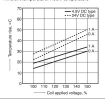
7. Ambient temperature characteristics Tested sample: AGQ200A4H, 6 pcs.
