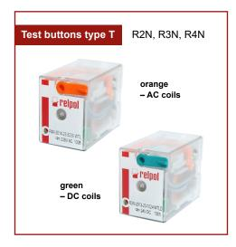
**Test buttons (no latching)** are recommended for R2N...WT, R3N...WT, R4N...WT, R15...WT 2 CO, R15...WT 3 CO relays - **for applications that do not allow permanent contact latching**. By manual operation (pressing the button) relay contacts can get switched for as long time as long the button is pressed. Contacts return to initial position as soon as pressure is released from the button. Those operations can be done while the coil is deenergized **6**.
