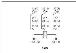
Note: the indicated polarity of the supply refers to the relays with extra equipment  $\boldsymbol{\mathsf{D}}$  - surge suppression element (diode) - for DC coils only.
