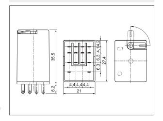
**Dimensions** - plug-in version, with test button (no latching) or with plug (no manual operation)
