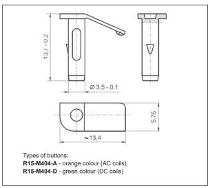
Plugs R4W-0003 or R15-M203 can substitute button type T if manual operation (latching and testing) is not allowed. Changing button type T for plug can be done by Customer themselves in the same way as changing button type T for button (no latching).
