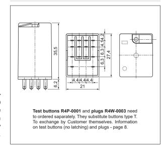
**Dimensions** - PCB version (WT), with lockable front test button type T
