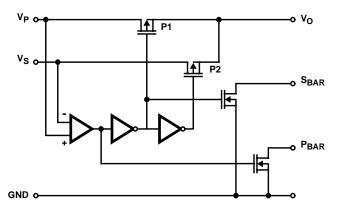
$V_{P}$  >  $V_{S},$  P1 SWITCH ON AND  $P_{BAR}$  SWITCH ON  $V_{S}$  >  $V_{P},$  P2 SWITCH ON AND  $S_{BAR}$  SWITCH ON
