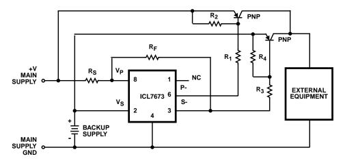
FIGURE 13. HIGH CURRENT BACKUP SYSTEM WITH HYSTERESIS
