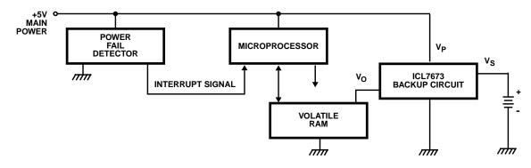
FIGURE 10. TYPICAL MICROPROCESSOR MEMORY APPLICATION
