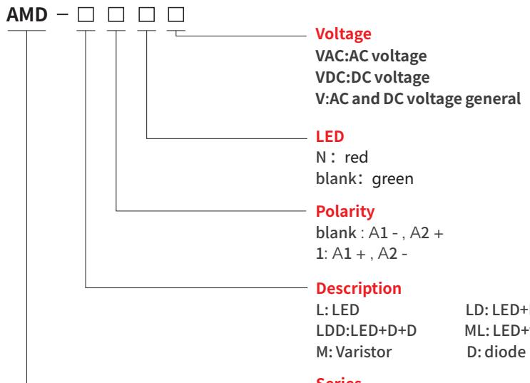
◆ For surge suppressor      ◆ With LED      ◆ Work with relay socket
