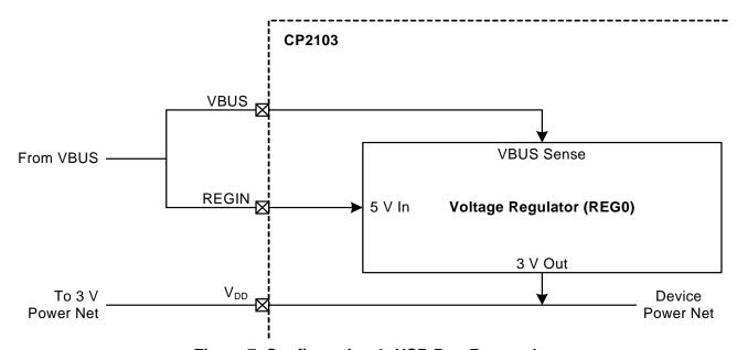
Figure 7. Configuration 1: USB Bus-Powered
