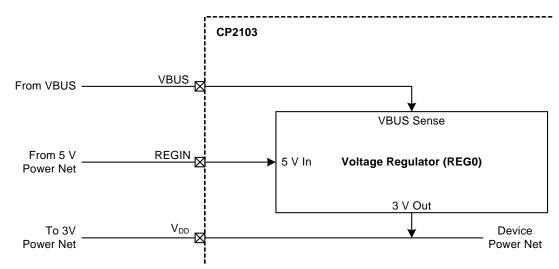
Figure 8. Configuration 2: USB Self-Powered
