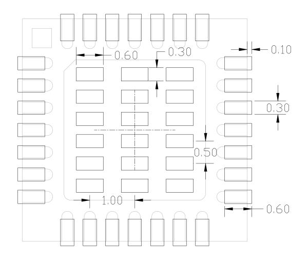
Figure 5. Typical QFN-28 Solder Paste Diagram
