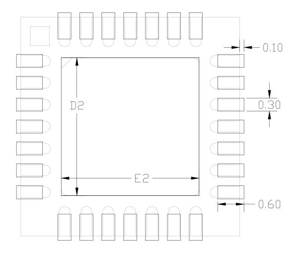
Figure 4. Typical QFN-28 Land Pattern
