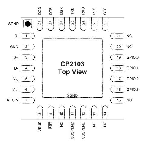
Figure 2. QFN-28 Pinout Diagram (Top View)
