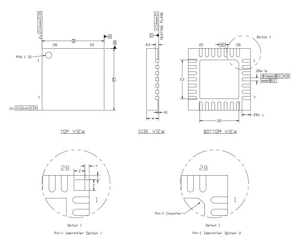
Figure 3. QFN-28 Package Drawing
