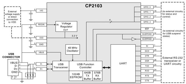
Figure 1. Example System Diagram
