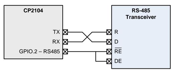
Figure 6. RS-485 Transceiver Typical Connection Diagram
