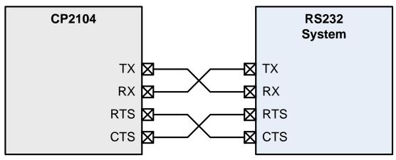
Figure 7. Hardware Flow Control Typical Connection Diagram
