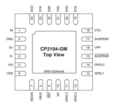
Figure 2. QFN-24 Pinout Diagram (Top View)
