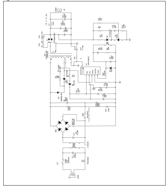
Figure 2. Electrical schematic
