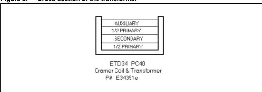
The transformer is wound with a split primary to reduce leakage inductance and minimize the snubbing needed. The auxiliary winding is placed on the outside to achieve the coupling needed for the current limiting function.
