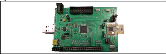
The STEVAL-SPZB260Vx is a demonstration kit of the SPZB260-PRO series of ZigBee modules that enables you to test ZigBee protocol feature capabilities and to prototype a coordinator, a router or an end device for your target ZigBee application. It includes a development board and a package of software libraries.
