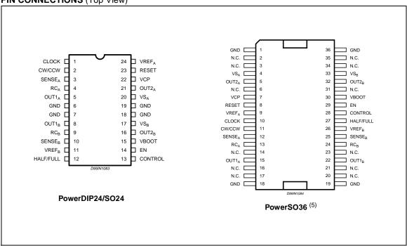
(5) The slug is internally connected to pins 1,18,19 and 36 (GND pins).
