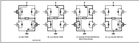
Figure 15. Slow Decay Mode Output Stage Configurations
