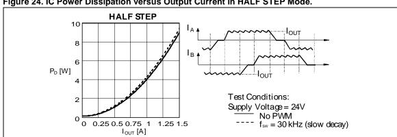
Figure 24. IC Power Dissipation versus Output Current in HALF STEP Mode.
