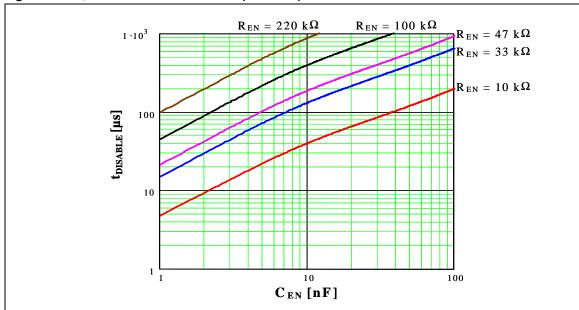
Figure 21. t<sub>DISABLE</sub> versus C<sub>EN</sub> and R<sub>EN</sub> (V<sub>DD</sub> = 5V).
