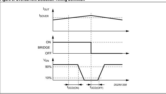
Figure 5. Overcurrent Detection Timing Definition
