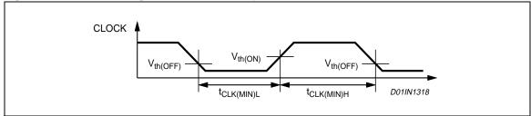
Figure 4. Minimum Timing Definition; Logic Inputs
