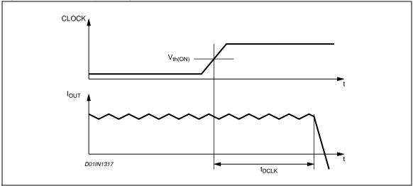
Figure 3. Minimum Timing Definition; Clock Input
