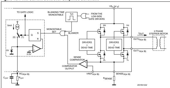
Figure 10. PWM Current Controller Simplified Schematic
