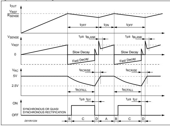
**Figure 11. Output Current Regulation Waveforms**
