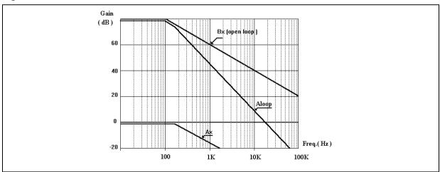
The BODE diagram shows together the error amplifier open loop transfer function, the Ax function and the resultant total Aloop given by the following equation :
