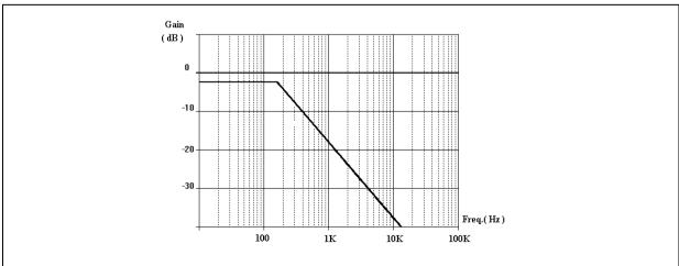
The Bode plot of the AxIdB function shows a DC gain of -1.9dB and a pole at 163Hz.
