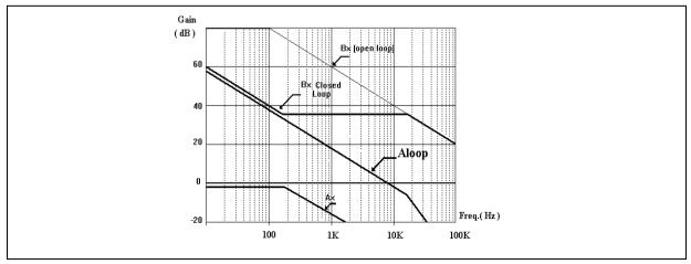
We can see that the effect of the load pole is cancelled by the zero of the Bx block ; the total Aloop cross a the 0dB axis with a slope of -20dB/decade, having in this way a stable system with an high gain at low frequency and a bandwidth of around 8KHz.
