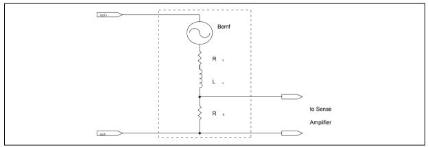
The schematic now shows the equivalent circuit of the stepper motor including a sine wave voltage generator of the Bemf. The Bemf voltage of the motor is not constant, its value changes depending on the speed of the motor.
