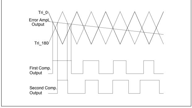
In the case of  $V_{DAC}$  equal to zero, the transconductance loop is balanced at the value of Vr, so the outputs of the two comparators are signals having the same phase and 50% of duty cycle.
