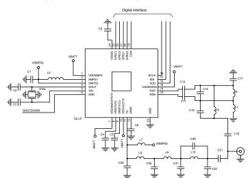
Figure 2. Suggested application diagram (embedded SMPS used)
