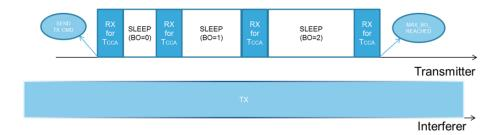
Finally, if the channel becomes free (for example during one of the SLEEP times), the device must assert channel free for a number of **NUM.\_OF\_CCA\_PERIOD** (T. listen) before transmitting:
