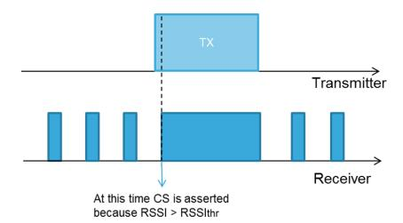
Figure 21. Fast Rx termination: CS detection
