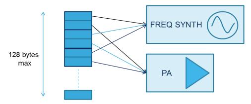
As for the normal TX operations, the TX\_FIFO samples are consumed and a management of the TX\_FIFO\_THRESHOLD is needed to perform transmissions longer than 128 samples.
