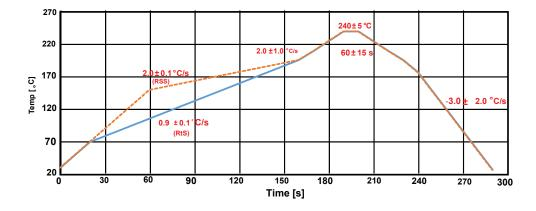
Figure 32. QFN recommended soldering profiles
