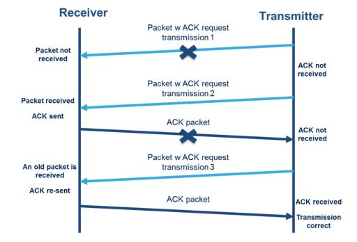
Figure 15. Automatic retransmission scenario
