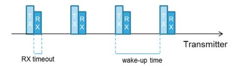
On each wake-up slot, the S2-LP enters TX only if the TX-FIFO is not empty, otherwise the TX slot is skipped with the device remaining in SLEEP.
