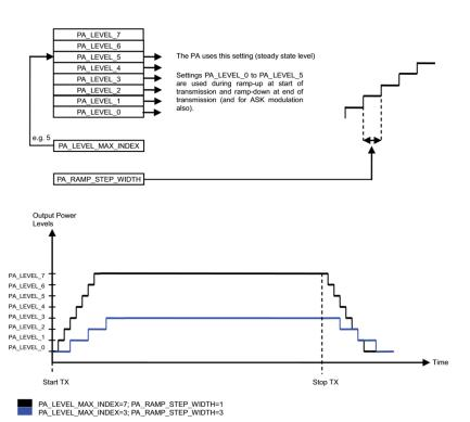
Figure 10. Output power ramping configuration
