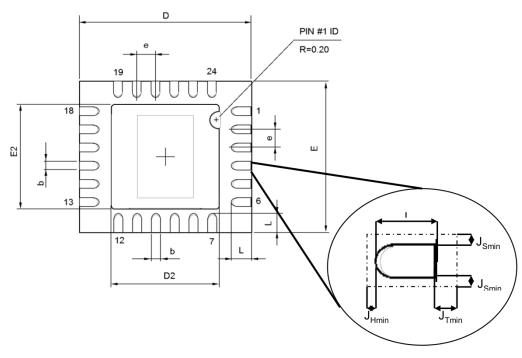
Figure 31. QFN24 4x4x1pitch 0.5 mm PCB pad pattern
