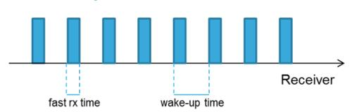
Figure 20. Fast RX termination mode with LDC
