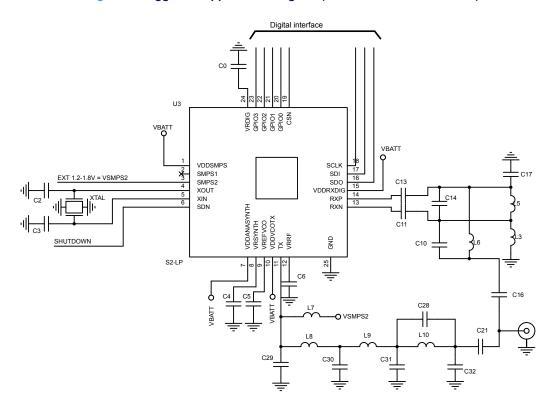
Figure 3. Suggested application diagram (embedded SMPS not used)
