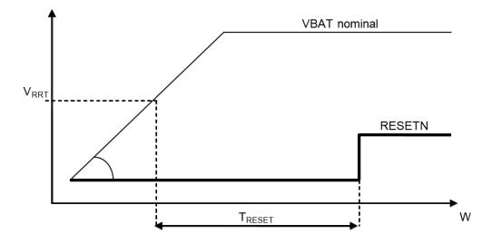
Figure 6. Power-On-Reset timing and limits
