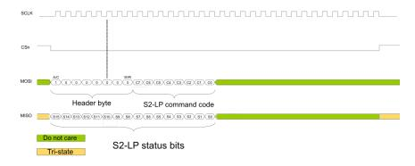
Concerning the first byte, the MSB is an A/C bit (address/commands: 0 indicates that the following byte is an address, 1 indicates that the following byte is a command code), while the LSB is a W/R bit (write/read: 1 indicates a read operation). All other bits must be zero.
