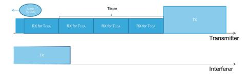
If the channel is busy and persistent\_mode bit is 0, the device will check the channel for the Tcca period. At the end, being the CS (carrier sense) signal high, it will switch in SLEEP for a randomic time that can last  $BO_{time} = T_{RCO}^* (6 + \text{rand}(0 : 2^{(NB+1)})^* (BU_{PRESC} + 1))$  with NB=0
