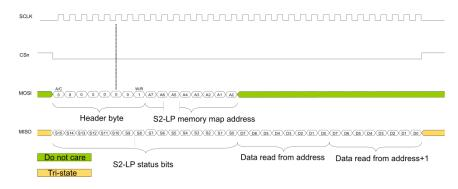
Figure 29. SPI command sequence
