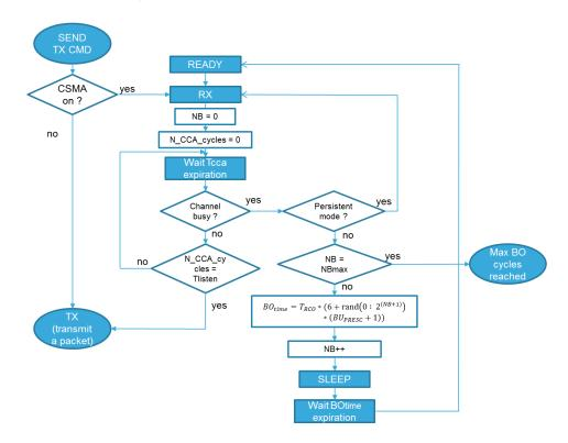
Figure 22. Flowchart of the S2-LP CSMA procedure
