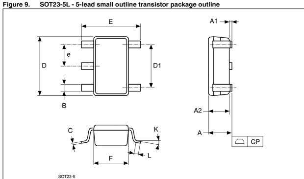
Table 4. SOT23-5L - 5-lead small outline transistor package mechanical data
