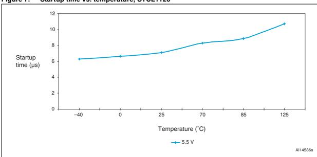
Figure 7. Startup time vs. temperature, STCL1120
