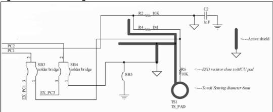
To disable the touch sensing interface and to use PC1, PC2 and PC3 as standard I/O, you need to unsolder the 2-1 connection and solder 2-3 connection on SB4 and SB3, you also need to unsolder the R2 resistor.
