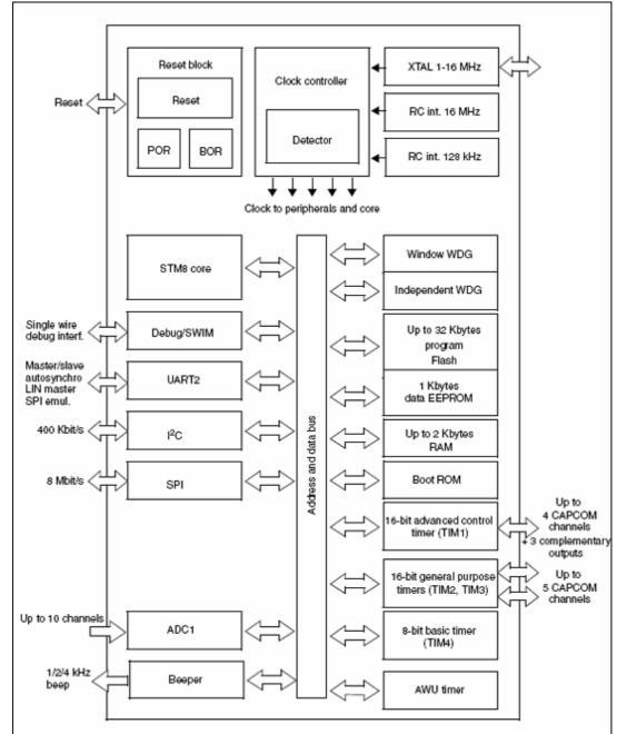
Figure 5. STM8S105 block diagram
