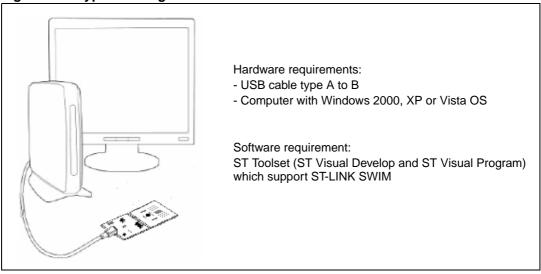
Note: The driver for ST-LINK is installed automatically when the USB is connected.
