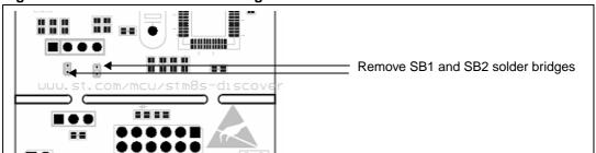
Figure 8. Separated ST-LINK module
