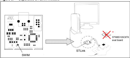
Warning: By removing this module you will lose power supply on the STM8S105C6T6 evaluation board. In consequence, you will not be able to program and use the STM8S105C6T6 board without a SWIM cable and an external power supply.
