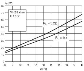
Figure 6: Output Power vs Supply Voltage (@  $R_L = 4\Omega$ )
