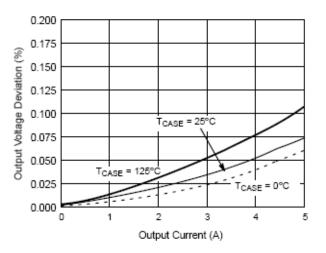
Figure 3. Load Regulation vs. Output Current
