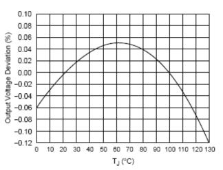
Figure 2. Reference Voltage vs Temperature
