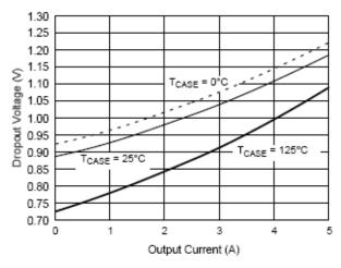
Figure 1. Dropout Voltage vs Output Current
