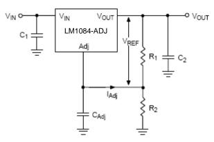
Figure 8. Resistor Divider Scheme for the Adjustable Version
