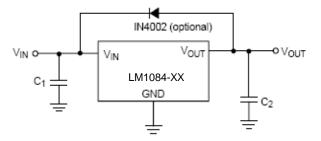
Figure 9. Protection Diode Scheme for Fixed Output Regulators
