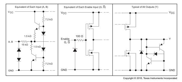
Figure 8. Schematics of Equivalent Inputs and Outputs
