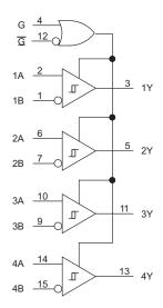
Figure 7. Logic Diagram (Positive Logic)
