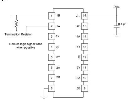
Figure 21. Layout With PCB Recommendations
