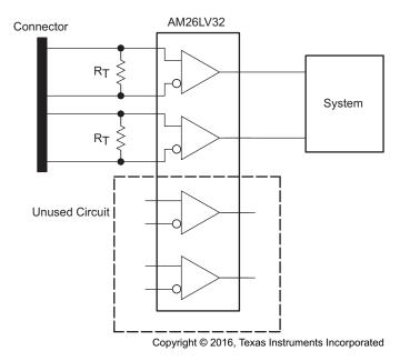
Figure 14. Typical Application With Unused Receivers
