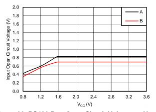
Figure 20. RS422 Port Open-Circuit Voltage vs  $V_{\rm CC}$
