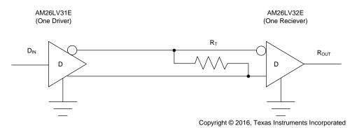
Figure 19. Differential Terminated Configuration
