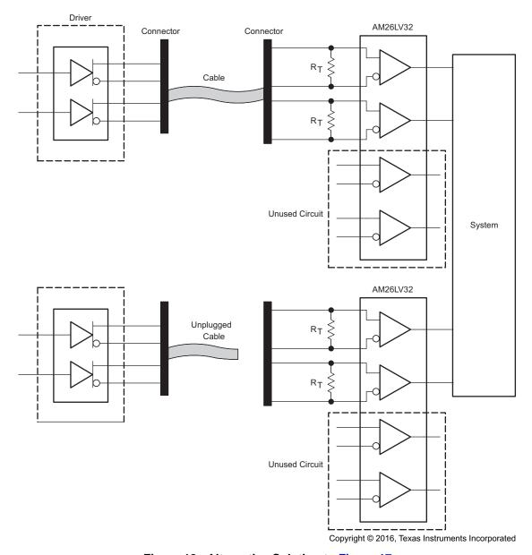
Figure 18. Alternative Solution to Figure 17
