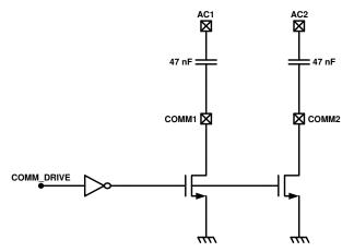
Figure 8-11. Capacitive Load Modulation
