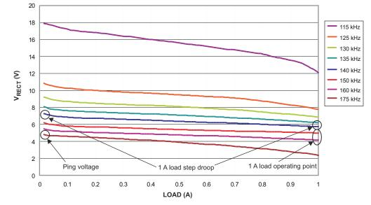
Figure 8-17. Example Load-Line Results
