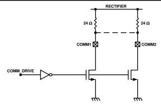
Figure 8-10. Resistive Load Modulation
