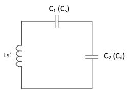
Figure 9-2. Dual Resonant Circuit With the Receiver Coil
