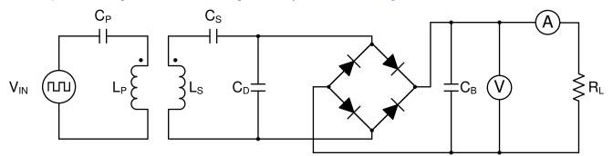
Figure 8-16. Load-Line Analysis Test Bench
