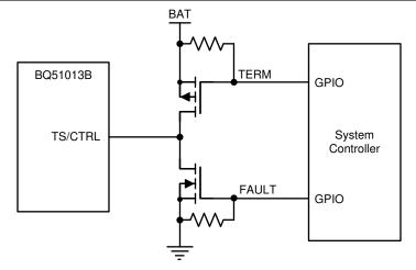
Figure 8-15. 3-State Driver For TS/CTRL
