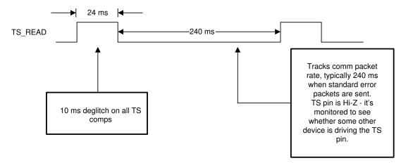
Figure 8-14. Timing Diagram For TS Detection Circuit
