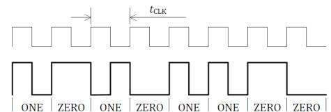
Figure 8-7. Differential Bi-Phase Encoding Scheme (WPC Volume 1: Low Power, Part 1 Interface Definition)
