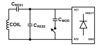
Figure 8-5. Capacitive Modulation
