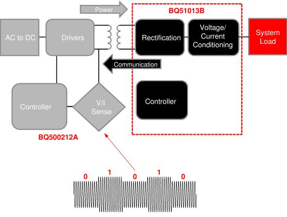
Figure 8-6. TX Coil Voltage/Current
