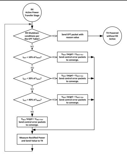
Figure 8-3. Active Power Transfer Flow Diagram
