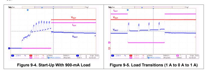
Figure 9-5 shows a current transition. The plot shows a 1-A load removed then added again. Note the stability of  $V_{OUT}$ .
