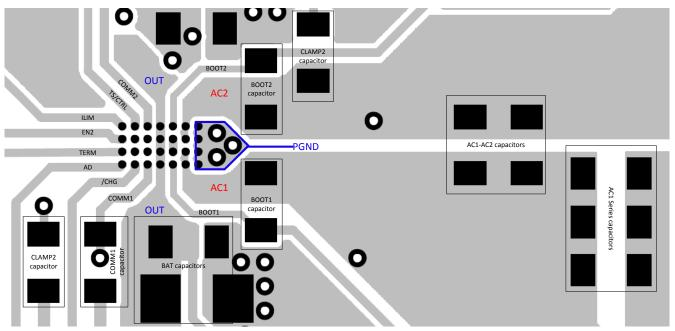
For the RHL package, the thermal pad should be connected to ground to help dissipate heat.
