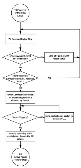
Figure 8-2. Wireless Power Start-Up Flow Diagram
