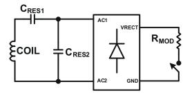
Figure 8-4. Resistive Modulation
