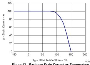
Figure 12. Maximum Drain Current vs Temperature
