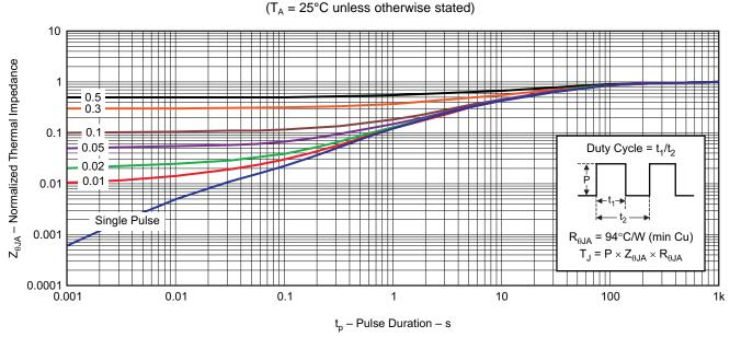
Figure 1. Transient Thermal Impedance
