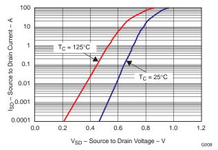
Figure 9. Typical Diode Forward Voltage
