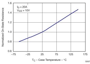
Figure 8. On Resistance vs Temperature
