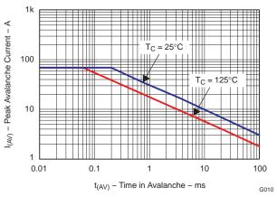
Figure 11. Single Pulse Unclamped Inductive Switching
