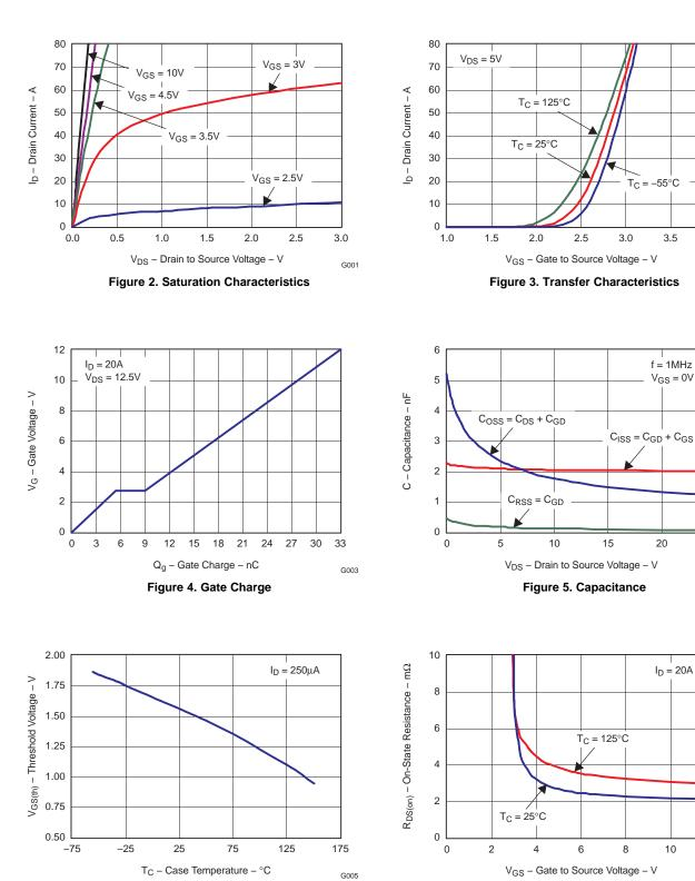
Figure 7. On Resistance vs Gate Voltage
